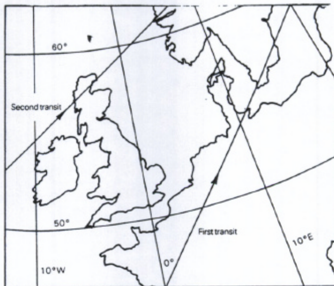
Figure 7: 90 Minute Orbit Tracks at 65° Inclination (U)
